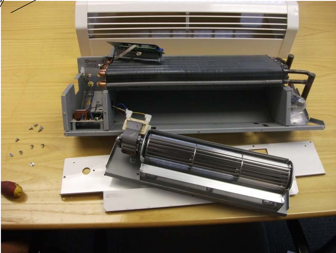
Motor tabs. Bend up slightly to release. The motor will lift out complete with the mounting plate.
