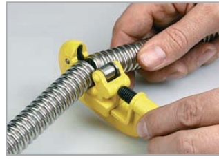
Cut pipe with tubing cutter. Do not use a hack saw.
