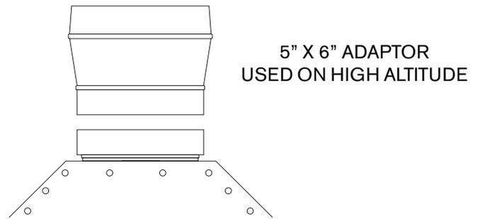
**Fig. 4 - Vent Adaptor for High Altitude Installations**
