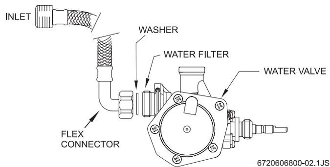
Fig. 6 - Water valve and water connector, top view
