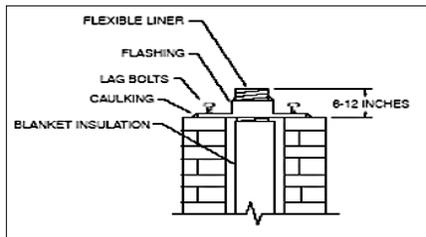
Chimney Flashing over the liner and secure it to chimney top using suitable anchors. Using a quality high temperature sealant, caulk all joints and paint if necessary.
