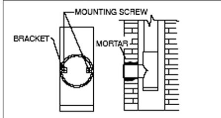
through the attached brackets. Using a standard mortar mix, cement around the horizontal portion of the Base Tee at the inlet opening.
