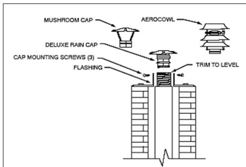
or Mushroom Cap or Aerocowl, and secure it with three (3) screws to the Flashing.
