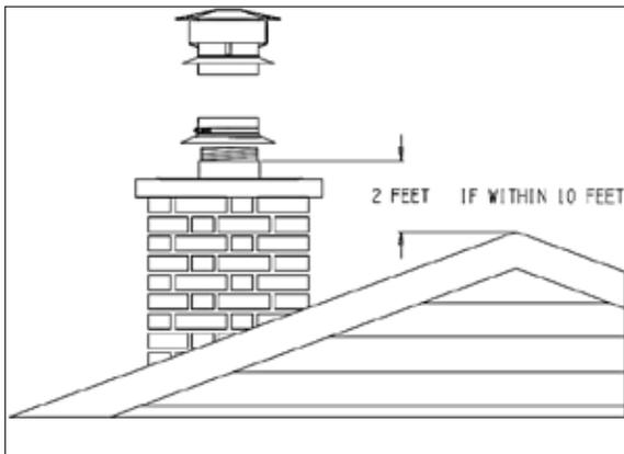
The air space clearance between the masonry chimney exterior and combustible materials should be checked to verify that the chimney is in accordance with the clearance specifications contained in the NFPA 211 Standard or other recognized major building codes, i.e., on an exterior chimney, clearance is 1" while on an interior chimney, clearance is 2".
