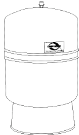
TV Expansion Tank
